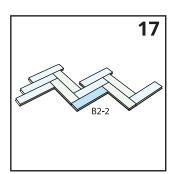
5. After installing these panels, you can start creating the next 'V-row' with a new supporting (B)panel and follow then repeat the above steps. It is very important to make sure the rows are perfectly centered in the middle of the room.
