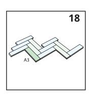
Step 9. After having installed about 5 full V-rows, you can take away the supporting (B) panels and move the rows up to the starter wall, as shown in figure 20. Don't forget to take into account an expansion gap between the wall and the panels. Step 10. The open triangles between the starter wall and the installed V-rows still need to be installed.
