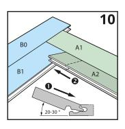
groove of panel (B0) at an angle of about 20-30 degrees. Slide panel (B1) until the tongue on the short side is positioned just above the groove of panel (A1), then press panel (B1) down to ensure the long sides of panels (B1) and (B0) are connected. Finally connect the tongue on the short side of panel (B1) by making use of the rubber hammer, in the same way as described above. See figures 6-8.
