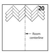
installation. The marked panel can now be sawn. Insert the long sides of the cut-off panels at an angle of about 20-30 degrees. Press the panels down to ensure these long sides
